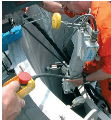
Ultrasonic device allows on-site inspection of annulus between inner and outer screens.
