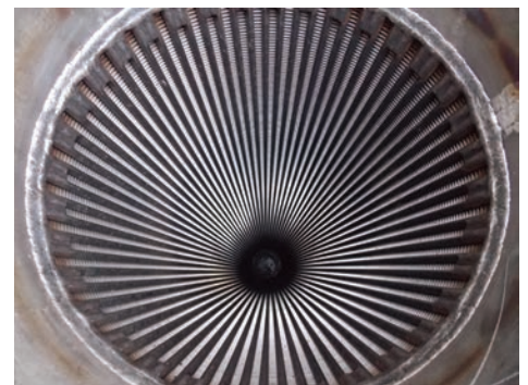
24 in. screen installed
