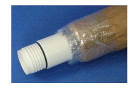
Materials Paper sleeve filled with silica sand and granular Bentonite
