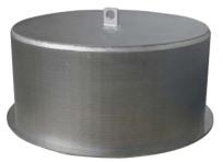
In downflow and upflow process applications, a screen at the bottom of the vessel is required to prevent media from migrating out of the vessel and to provide proper upflow distribution of the process gas or liquid. This function is best performed with a Johnson Screens' Vee-Wire® outlet basket.
