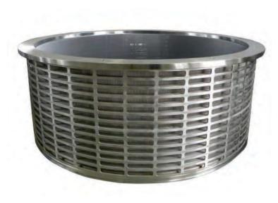
Johnson Screens' caged screens are designed to work in harsh environments. These screens use a reinforced stainless steel cage and are designed to give more rigidity and strength than other designs. Using a steel webbed structure, creates force multiplying strength to the rings and a stiffeners to reduce moments of inertia. With this design, Johnson Screens' caged screens distribute the pressure drops over a larger area of the structure increasing life and longevity.
