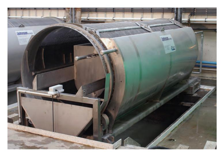
Johnson Screens' EMD Rotary Drum Screen are installed at a 35° angle and are used for trash screening and water treatment in the pulp and paper industry. These screens can be used for fine or coarse screening applications. This is a self-contained single unit. The screen drum is constructed out of Vee-Wire, however, perforated plate and mesh designs are also offered. EMD Rotary Drum Screen can also be installed either directly in the channel or in a separate tank.
